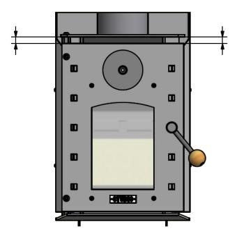
Check both ends of the doors to make sure it is parallel to the unit.
