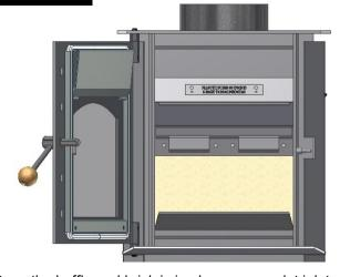
Once the baffle and brick is in place, ensure jet inlet holes on the back plate are clear of any obstructions.
