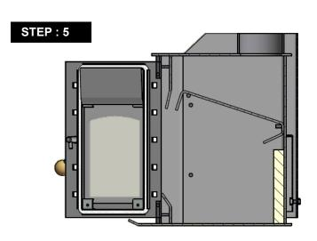
Push the baffle back so it rests on the support pins on the sides and the firebox back.
