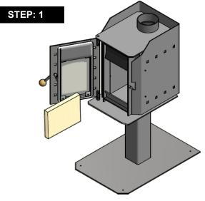
Place vermiculite board back brick into the back of the Firebox.
