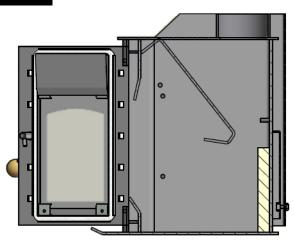
Push the baffle up to the top of firebox.
