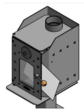
Nip up screws while holding door in place, then tighten fully with a 5mm allen Key.
