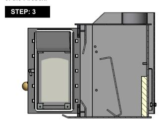
Straighten the steel baffle horizontally,
