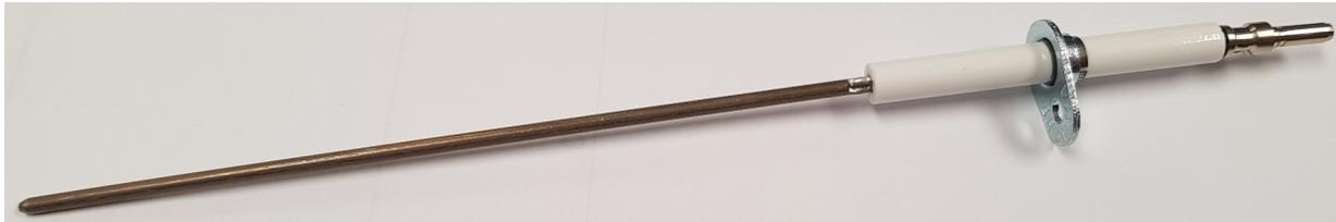
In most situations, a new probe will not work on your Warmington unit, and hence you will have to cut and bend to fit your specific unit. Care needs to be taken not to break the ceramic part of the probe. We suggest using two pliers to bend the metal rod, which will prevent damage to the ceramic component, see photo below for an example.
