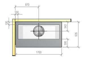
Warmington Gas Open Fire SG 1100 Freestanding Aspiring Cabinet - Straight Hearth Fire, Flue System to Comply with NZS 5261 / 5262 : 2003
