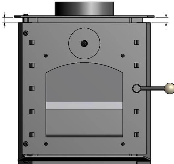
Check both ends of the doors to make sure it is parallel to the unit.
