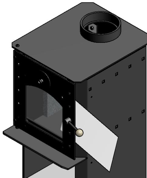
Nip up screws while holding door in place, then tighten fully with a 5m allen key.
