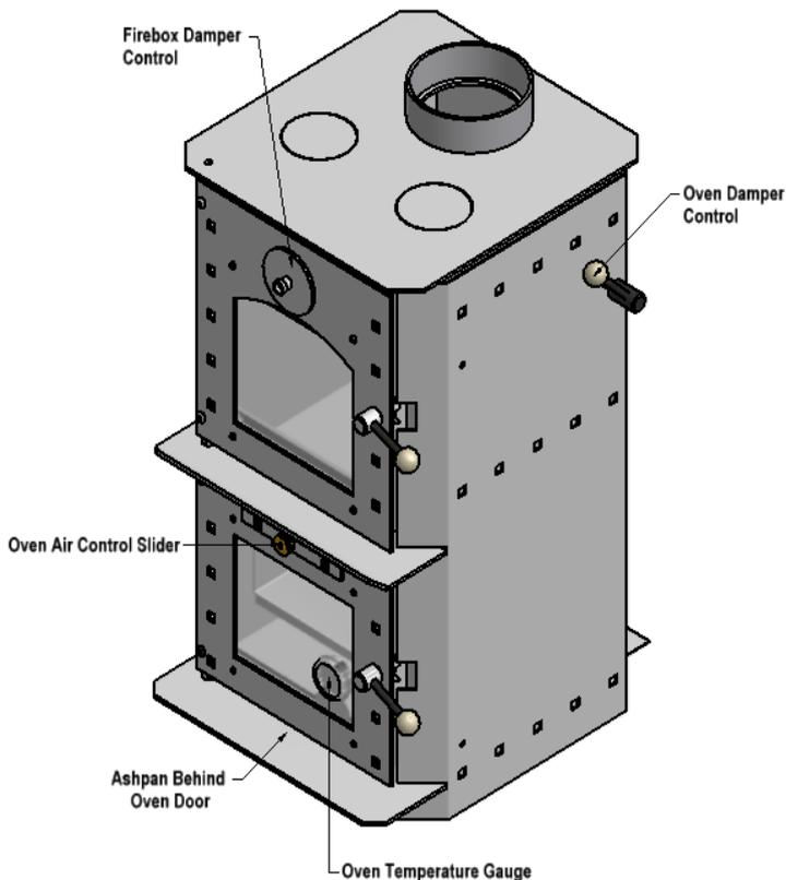
The Oven is heated directly by the Fire. In order to heat up the oven, the Fire should be lit as described in our Specifications. Once the Fire is established, pull the Oven Damper handle Forward. This will allow the Hot Fumes from the Fire to circulate around the Inner cavity thus heating up the Oven.
