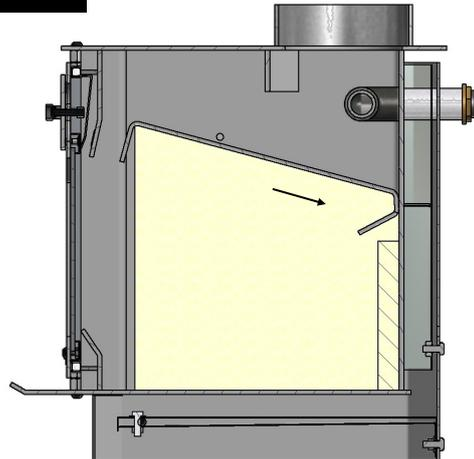
Push the baffle right to the back of firebox.
