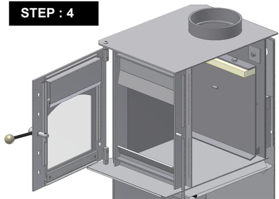
Push baffle right to the back of firebox
