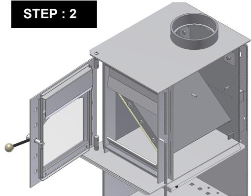
Tilt Studio baffle on an angle & slide in through door frame
