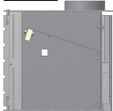
Move the back of the baffle up to sit on the pins at the back of the firebox
