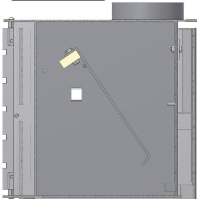
Move baffle forward to sit on pins
