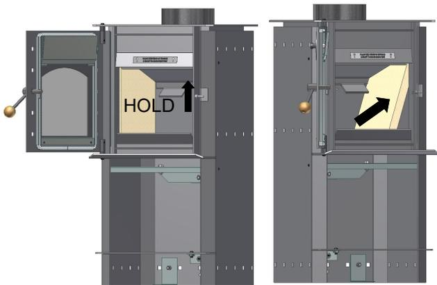
While holding up the steel baffle horizontally, insert the opposite side brick in from underneath it, as shown above. The 2 side bricks will now support the steel baffle.
