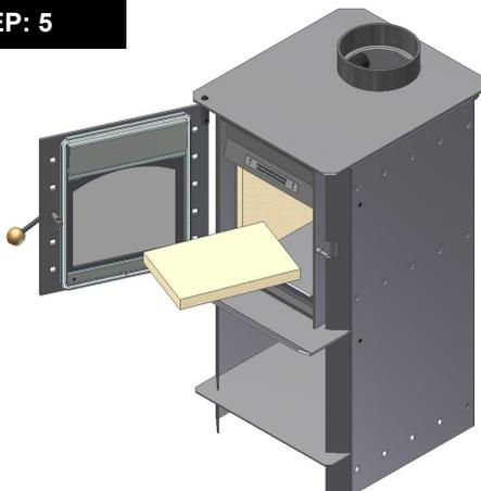
Fit back vermiculite board panel into the firebox back, ensuring that it is sitting hard against the back of the firebox.
